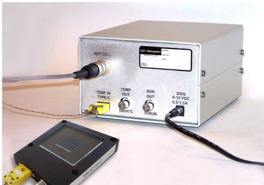
Figure 1: Connections made to the back of the meter
