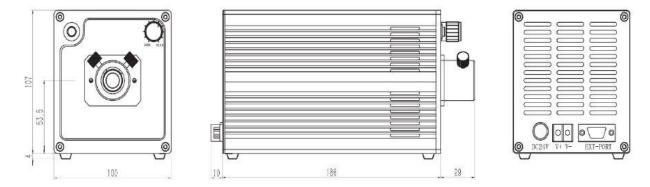
Figure 6: 66088-LED50 dimensions in mm.
