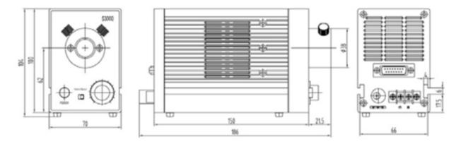
Figure 5: 66088-LED dimensions in mm.
