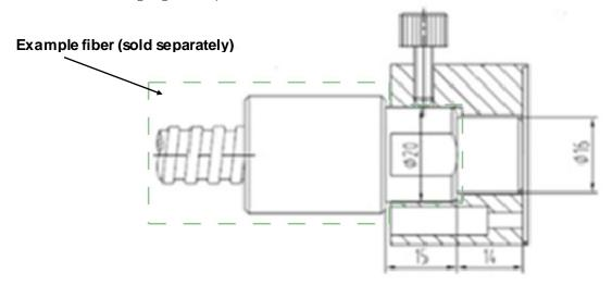
Figure 3: Interior dimensions (in mm) of the light guide socket.
