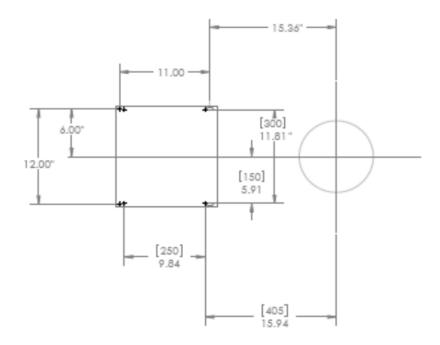
Figure 10: Base Plate Mounting Hole Locations Relative to Optical Centerline for 6x6 system
