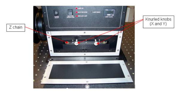
Photo 27: Lamp focus adjustment mechanisms (Access panel removed)
