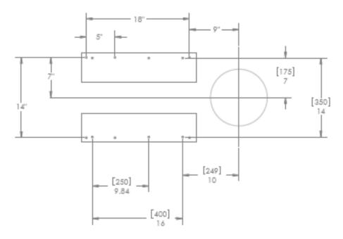
Figure 12: Base Plate Mounting Hole Locations Relative to Optical Centerline for 8x8 system
