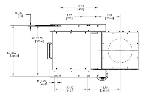
Figure 14: Base Plate Mounting Hole Locations Relative to Optical Centerline for 12x12 system
