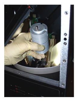
Photo 25: Heat sink unscrewed from socket
