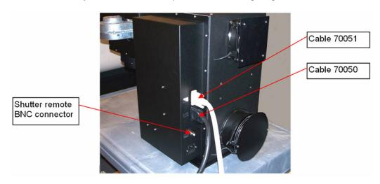
Photo 17: Electrical connections on simulator (black and gray cables)
