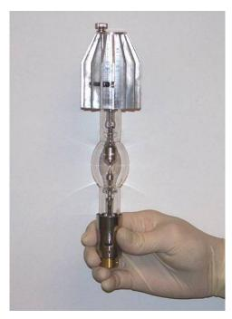
Photo 15: 1kW lamp with heat sink attached
