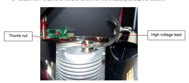
Photo 23: #10-32 thumb nut on heat sink
