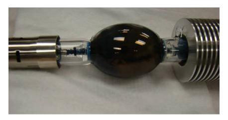
Photo 30: Lamp run under reverse polarity
