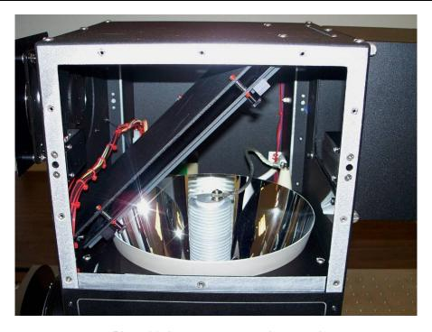
Photo 22: Lamp access panel removed
