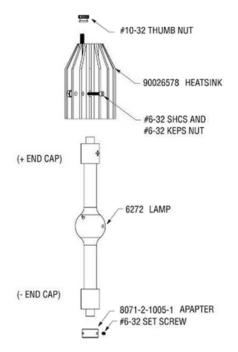
Figure 3: Lamp Assembly for 1kW Lamp
