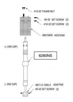
Figure 2: Installing the 450W Lamp
