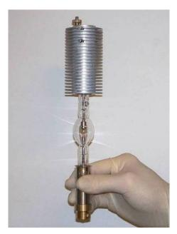
Photo 14: 450W Lamp with heat sink attached
