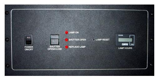
Photo 19: The illuminator housing control panel
