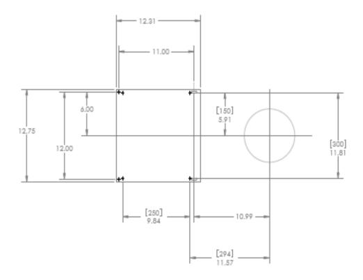
Figure 8: Base Plate Mounting Hole Locations Relative to Optical Centerline for 4x4 system
