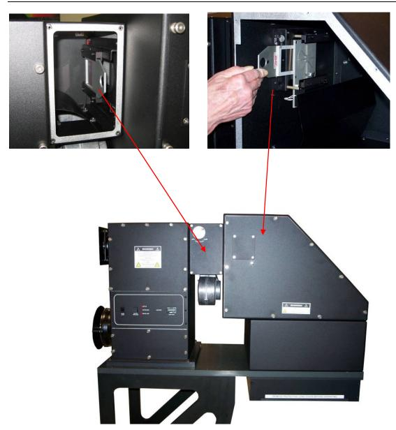
Proper installation placement of other Air Mass filters for various models (Same location as the standard AM1.5G for various models)
