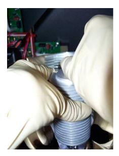
Photo 24: Removing the high voltage lead from the heat sink.
