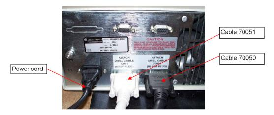
Photo 18: Electrical connections on power supply (black and gray cables)
