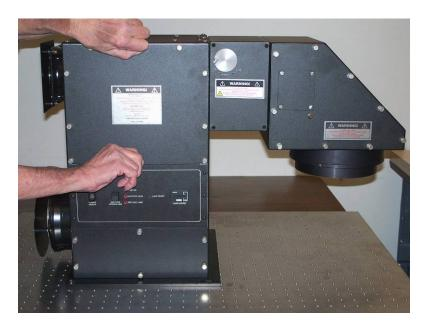
Photo 12: Removing the lamp access panel
