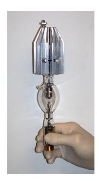
Photo 16: 1.6kW lamp with heat sink attached
