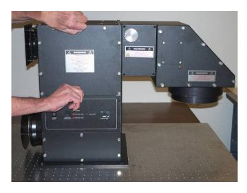
Photo 21: Removing the lamp access panel
