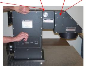
Air mass 1.5G filter installed **here** for 2x2 and 4x4 models
