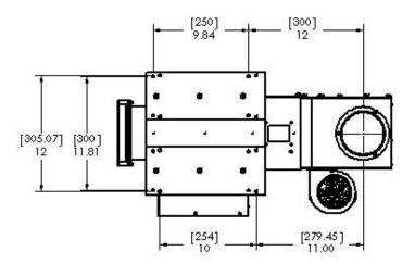
Figure 6: Base Plate Mounting Hole Locations Relative to Optical Centerline for 2x2 system
