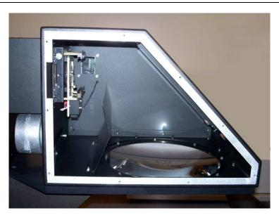
Photo 10: Output assembly, side cover removed
