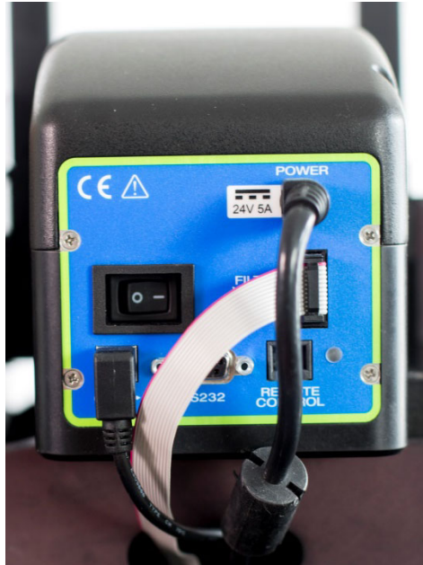
Monochromator Cable Connections
