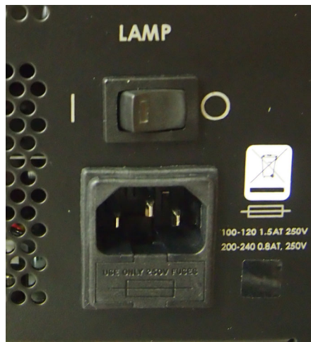
Lamp Power Switch and Connector
