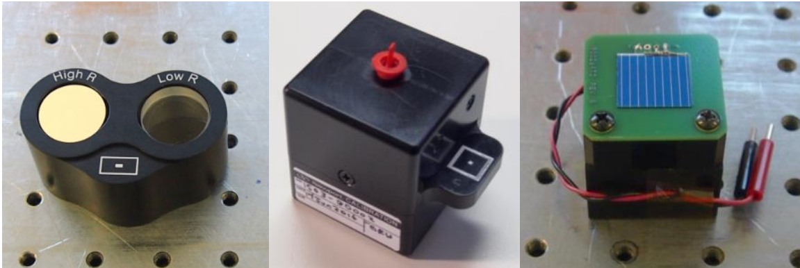
603414 Specular Reflectance Standard, 603621 Reference Detector, and SAMPLE-QESI Silicon Test Sample Cell
