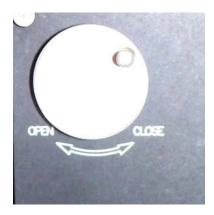
5. Turn on the power-supply and solar simulator. Adjust the knob in either direction to attain the desired output irradiance level. (Note: In order to attain the desired output, a reference cell or other irradiance measuring device should be used. Relying on the number of turns or knob orientation for any particular level of irradiance will not guarantee repetitive results. User will have to adjust the knob by measuring output irradiance, if a change in output irradiance is required.)
