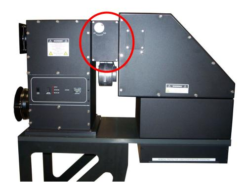
As shown above in the red circle, the partial sun attenuator fits in the middle section of the lamp housing for the applicable solar simulator models. The partial sun module comes with four Phillips pan head screws - black (6-32 x 3/8).
