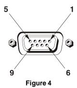
RS-232 Connector 9- Pin D-SUB Assignment
