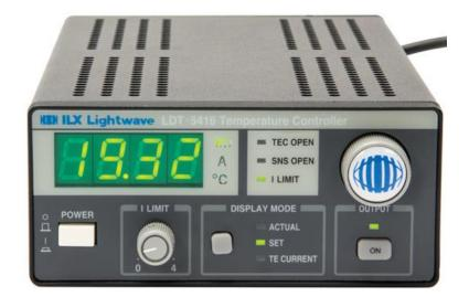
Figure 1.1 – LDT-5416 Front Panel
