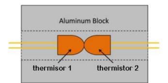
Figure 1: Internal view of the test load showing adjacent thermistors
