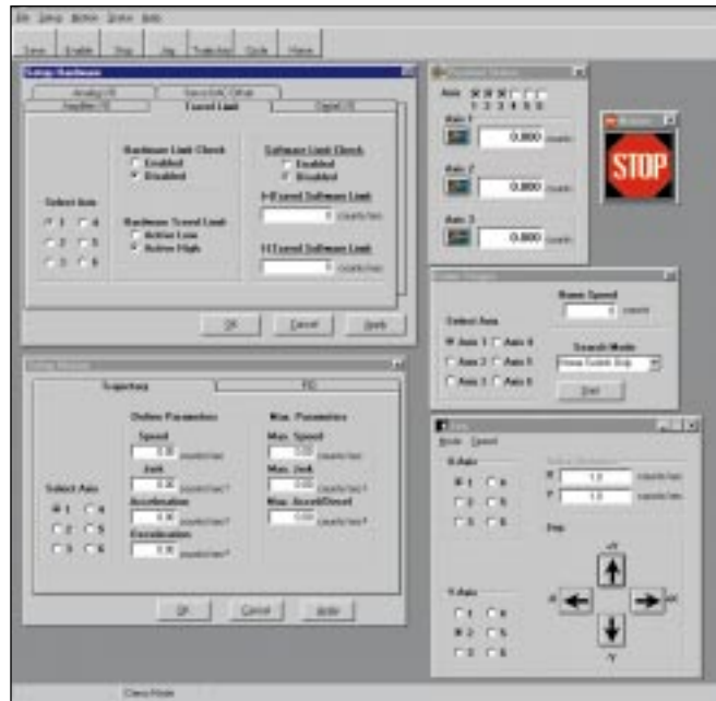
FIGURE 2. User interface for setting up and configuring the ESP motion control platform is Windows 95/NT-based. The graphical interface allows a user to intuitively configure the system within minutes.
