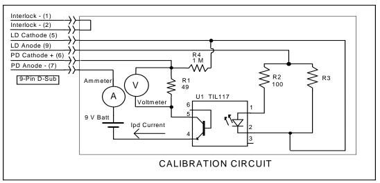
Figure 5.1 I<sub>PD</sub> Calibration Circuit
