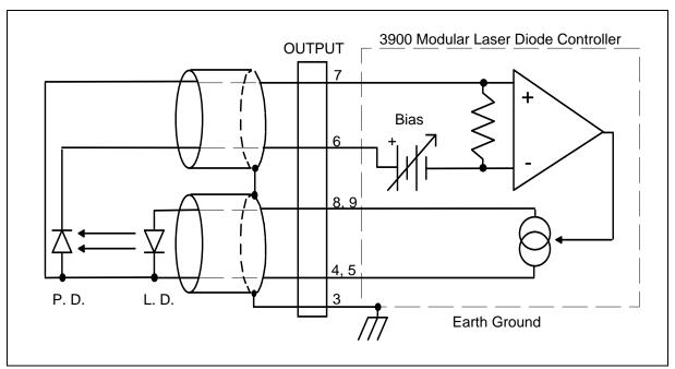
Figure 4.3B Common Laser Cathode - Photodiode Anode
