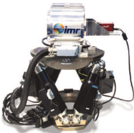
Figure 1: Optomechanical image derotator assembly on Newport HXP1000 (Courtesy of Universitat Hannover)
