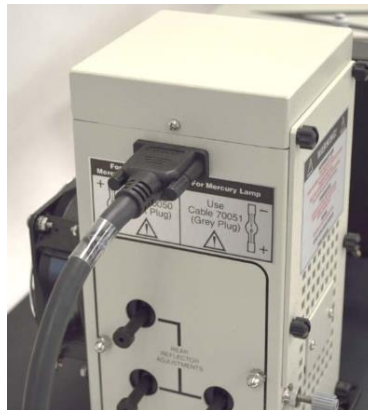
Figure 6 The electrical connector on an Oriel Research Lamp Housing for use with an OPS-A Model Power Supply.
