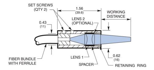
Lens 1 is a .5 diameter, 19 mm focal length, F/1.7 fused silica lens. The 77646 is shipped with this lens installed. This lens captures and collimates the diverging output from the fiber bundle.
