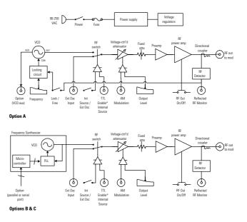
In the Option A configuration, a voltage-controlled oscillator (VCO) provides the sinusoidal frequency source. A front-panel knob controls the frequency by changing the applied voltage to the VCO. The main VCO output is the input to an RF switch, and an auxillary output is sent to the option port for monitoring.
