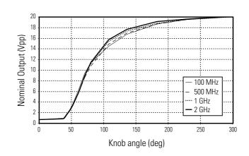
Figure 4: Output of RF Out in Vpp versus Output Level knob angle
