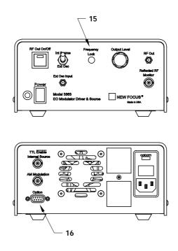
Figure 2: Front and rear panel of the 3363-B and 3363-C
