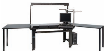
Figure 8. The new Vision IsoStation is available in multiple sizes from 24 × 24 up to 36 × 72 in. and two load capacities, 500 and 1300 lb. All models reduce transmitted vertical and horizontal vibrations by 70 percent (–10 dB) or more at 5 Hz and by more than 95 percent (–26 dB) at 10 Hz. The multiple storage and work surface options also help provide areas to store nonessential items or instrumentation that might otherwise induce vibrations.
