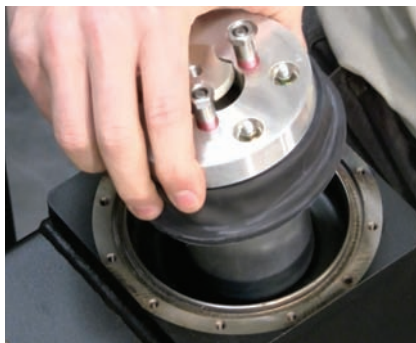
Figure 9. Choosing field-upgradable vibration control solutions like the SmartTable OTS platform isolator shown here can help meet near-term budgetary requirements and long-term performance needs.
