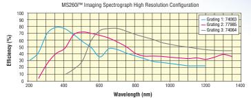
The efficiency curves above are relative (not absolute) and were measured using an in-plane near Littrow configuration. Please use the curves as a guide and not as absolute data.
