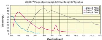
The efficiency curves above are relative (not absolute) and were measured using an in-plane near Littrow configuration. Please use the curves as a guide and not as absolute data.
