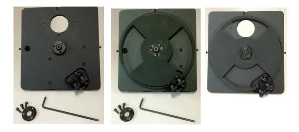
Insert the chopper wheel in the gap of the photodetectors and reattach the hub washer and screws.
