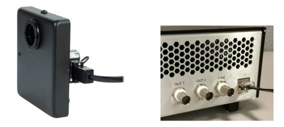
Install the chopper head in the desired location. The chopper head may be rotated in whichever direction is most convenient for connecting the cable to the chopper controller.
