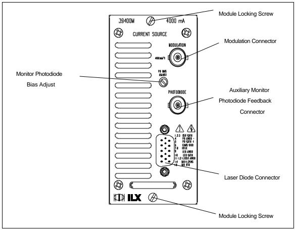
Figure 4.1 CSM-39400M Back Panel
