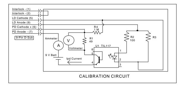
Figure 5.1 I<sub>PD</sub> Calibration Circuit
