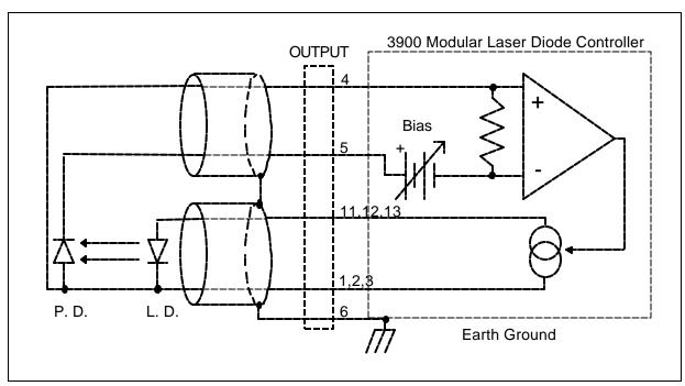
Figure 4.3B Common Laser Cathode - Photodiode Anode
