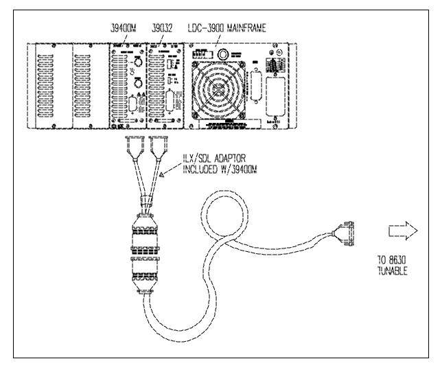
Figure 4.5 LDC-3900/Tunable Laser Configuration
