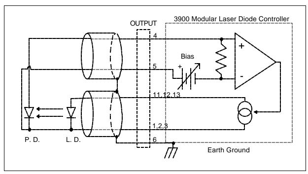
Figure 4.3A Common Laser Cathode - Photodiode Cathode
