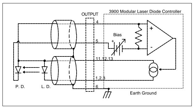
Figure 4.3D Common Laser Anode - Photodiode Anode
