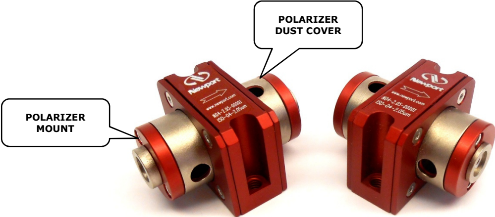
Figure 2: Overall view of a Newport 1µm ISO-FRDY Series Faraday Isolator
