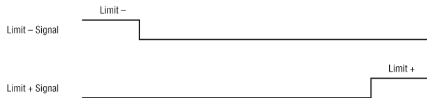
Figure 28: Limit - and Limit + TTL input signals.
