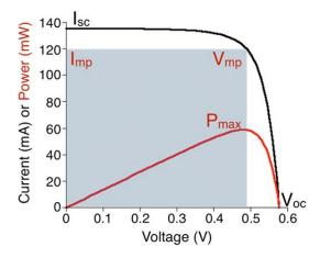
Figure 3 – A sample IV curve taken from a monocrystalline silicon PV cell (4 cm²) using the Oriel PVIV Kit.
