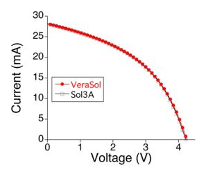
Figure 5b – VeraSol (red) and Sol3A (black) 1.0 sun IV curves from an amorphous silicon thin film module (6.75 cm<sup>2</sup>).
