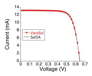
Figure 5a – VeraSol (red) and Sol3A (black) 1.0 sun IV curves from Copper indium gallium thin film PV cell (0.42 cm²).
