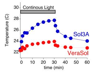
Figure 6c - PV cell temperature for the two experiments in A and B over the 30 minute light exposure as well as a 30 minute recovery with no light.
