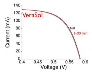
Figure 6A – IV Curves taken at 1, 3, 10, 15, 20, 30 minutes under continuous 1 sun illumination.
