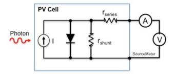
Figure 2– A simple diode circuit model describing a PV cell connected to a source meter for PVIV testing.
