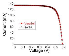
Figure 4 – VeraSol and Sol3A 1 sun IV curves from the calibrated monocrystalline silicon PV cell (number).
