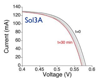
Figure 6b - IV Curves taken at 1, 3, 10, 15, 20, 30 minutes under continuous 1 sun illumination.
