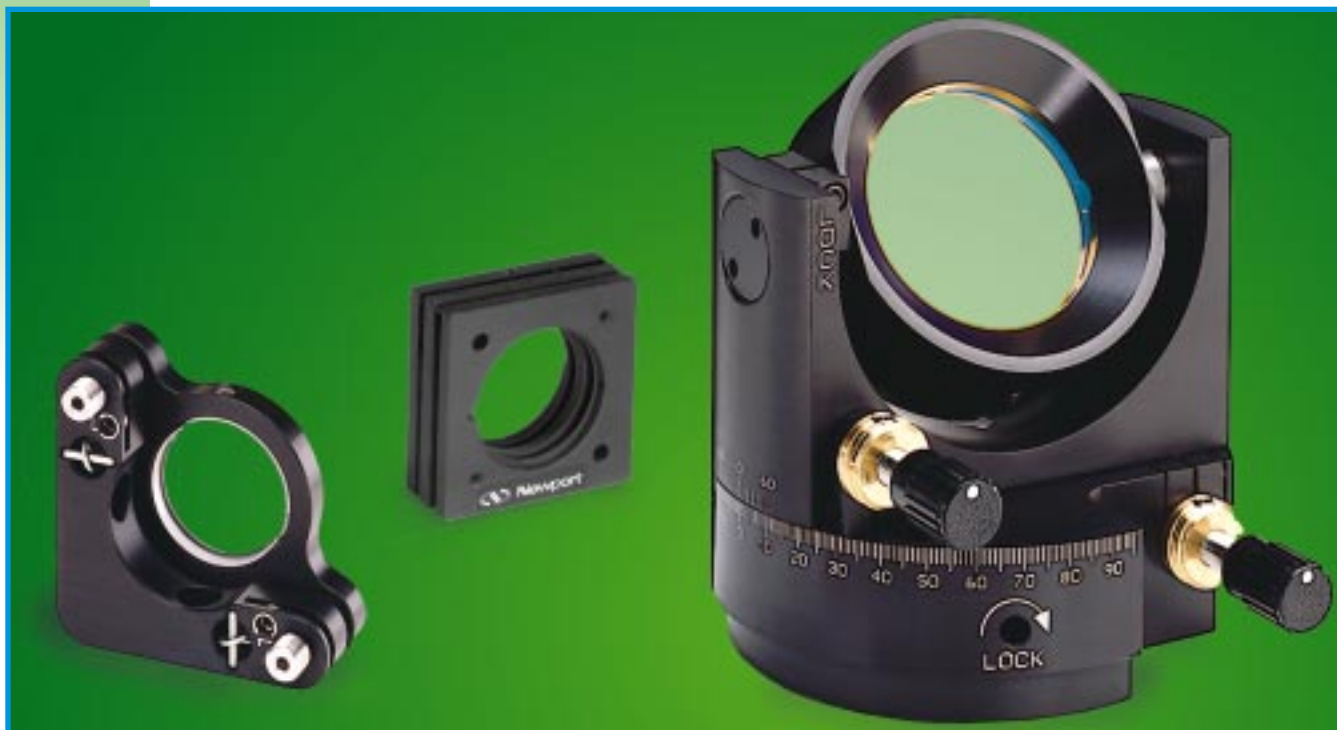
Figure 2. Three types of mounts with angular adjustments have advantages for different applications. “Cone, groove and flat” mounts (left) combine adjustment range and stability, and can be very economical. Flexure mounts (center) have more limited adjustment range but are compact, with excellent stability. Gimbal mounts have wide adjustment (up to 360 °) and a high load-bearing capacity.
