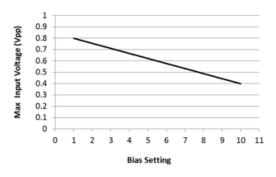
*Figure* 4. Maximum allowed peak–peak input voltage versus setting on the Bias Control Knob.
