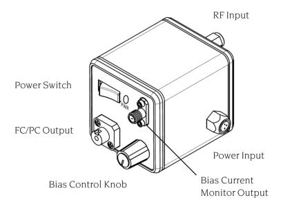
Figure 2. Connector and control descriptions.
