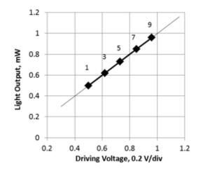
*Figure* 3. Typical light output versus driving voltage showing bias points.
