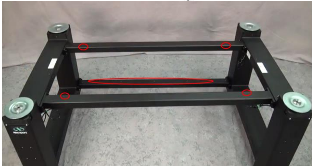
Figure 3 Leveling valve mounting holes located on the cross brace should be positioned inward and facing upward toward the top of the frame.
