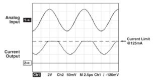
Each of the 3500B Series Current Sources feature a current limit "clamping" topology which prevents the limit from being exceeded under any condition including current modulation.
