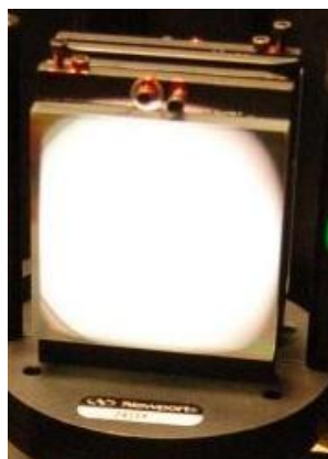
Figure 20: Grating Correctly “Filled” with Light
