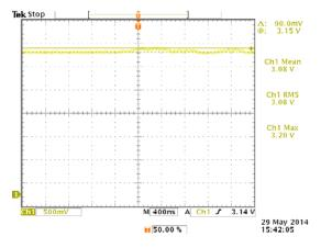
Figure 7: Effect on laser output due to 1 kV power surge event on AC power line
