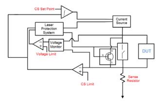
Figure 1: Schematic diagram of the LDC-3736 laser protection system circuitry
