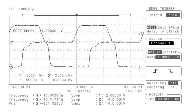
Figure 3. 20 MHz analog modulation for a laser operating at 635 nm.
