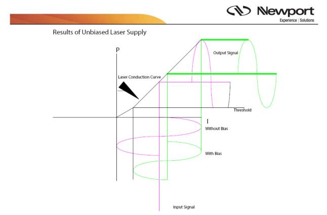
Figure 1. Modulation of input current and output power.
