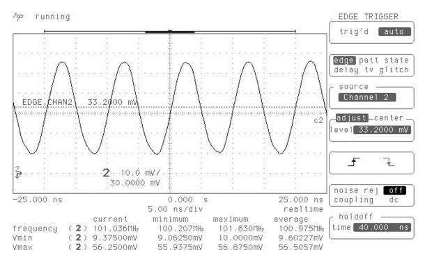
Figure 5 100 MHz TTL modulation for a laser operating at 405 nm.
