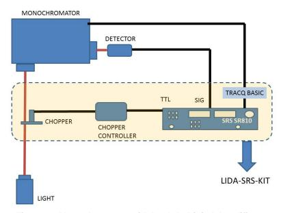
Figure 4: Monochromator with Lock-In Digital Amplifier
