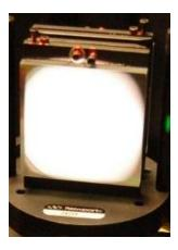
Figure 19: Grating Correctly "Filled" with Light
