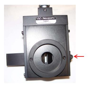
Figure 12: Tallest Micrometer Adjustable Slit Height
