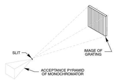
Figure 18: Acceptance Pyramid of Monochromator
