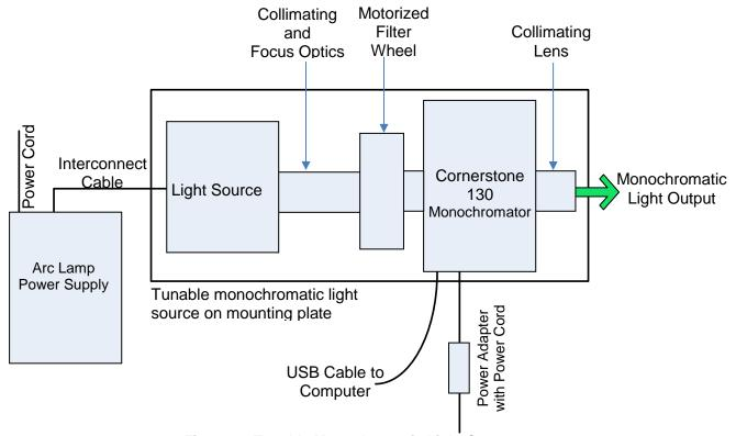
Figure 3: Tunable Monochromatic Light Source
