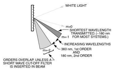
Figure 38: Polychromatic Light Diffracted From a Grating
