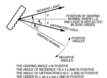
Figure 39: Sign Convention for the Angle of Incidence, Angle of Diffraction and Grating Angle
