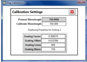
Figure 29: Entering Calibration Values in Utility Software
