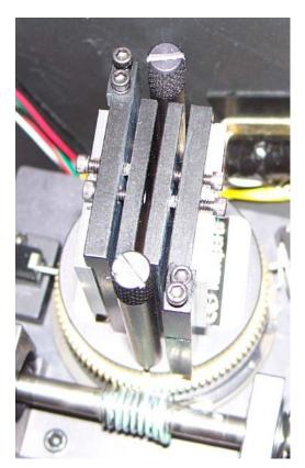
Figure 28: Grating Platform With Gratings Installed
