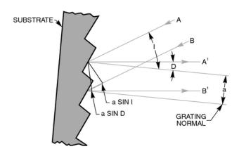
Figure 36: The Sawtooth Pattern of a Grating Section
