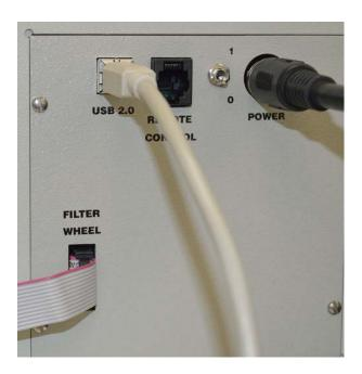
**Figure 6: Monochromator Connections**
