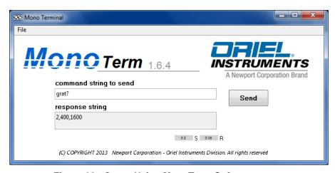
Figure 26: Query Using MonoTerm Software
