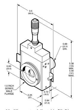
Figure 32: Micrometer Adjustable Slit Dimensions
