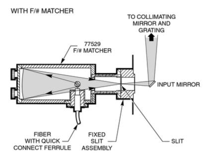
Figure 21: F Number Matcher Used with Fiber Optic Cable
