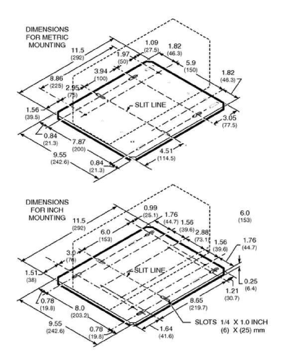
Figure 33: Model 74006 Mounting Plate
