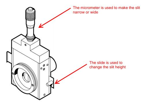
Figure 9: A Micrometer Adjustable Slit
