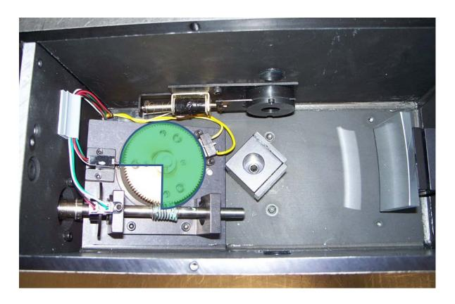
Figure 30: Grating Turret Position Sensor Pin Range
