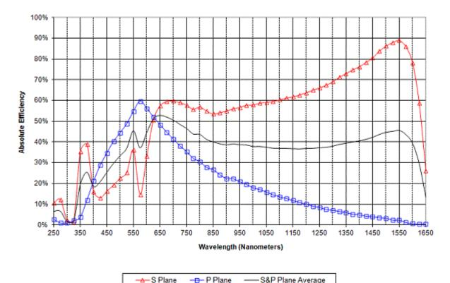
**Note:** The efficiency curve above is absolute and was measured in an in-plane near Littrow configuration (unless otherwise indicated). Efficiency curves are only representative: actual efficiency may vary significantly depending on use geometry and measurement technique. This efficiency curve is for master 5302; two masters with the same catalog number may have different efficiency curves. The uncertainty band on the data in the above efficiency curve(s) is +/- three percentage points.
