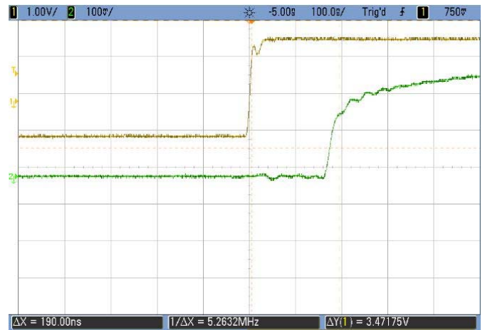
FIGURE 4: Trigger In to Optical Output Delay, 190ns
