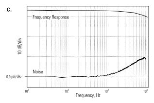
For the Model 2032 the bandwidth is  $900\,\mathrm{kHz}$  for the low gain setting and  $150\,\mathrm{kHz}$  for the medium and high gain settings.
