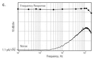
For the Model 2033 the bandwidth is 200 kHz for the low gain setting, 30 kHz for the medium gain setting, and 30 kHz for the high gain setting.
