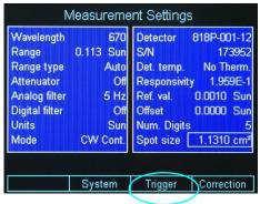
Figure 41 Accessing the Trigger Setup screen
