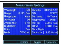
Figure 40 Measurement Settings screen
