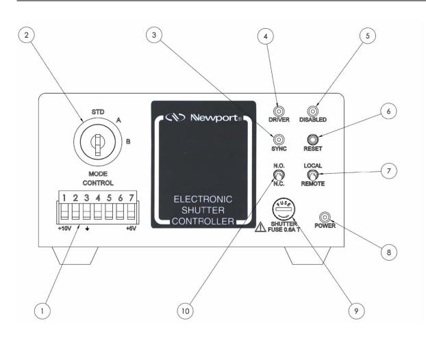
Figure 3: 76995 Front Panel Operator Controls
