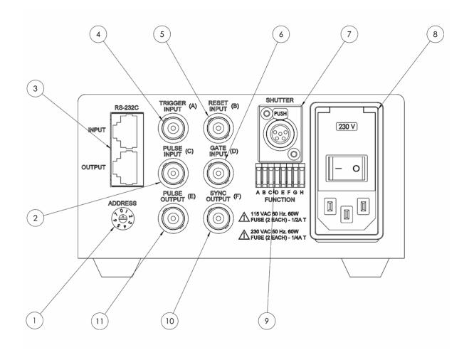
Figure 4: 76995- Rear Panel Operator Controls and I/O
