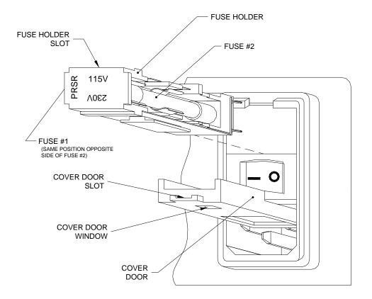
Figure 2: AC Input Module
