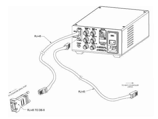
Figure 6: 76995 Daisy Chain Cable Configuration
