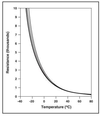
Figure 2. R-T slope changes for differing thermistor materials.
