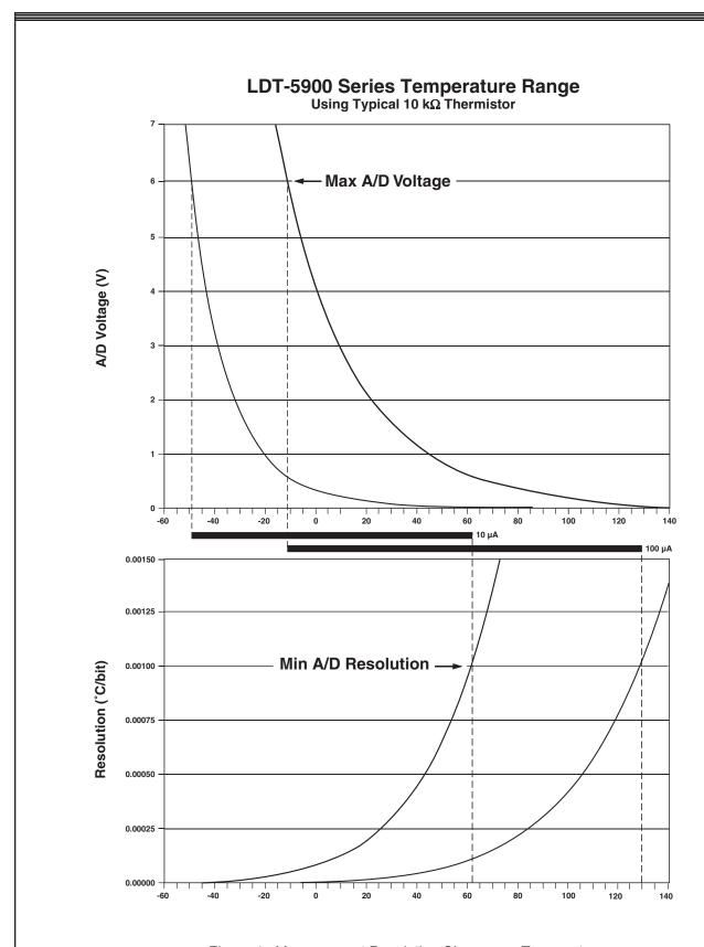
Figure 4. Measurement Resolution Change vs. Temperature
