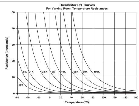
Figure 1. Resistance-Temperature response curves for nine common thermistors.
