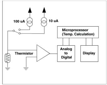
Figure 3. High resolution temperature measurement system.
