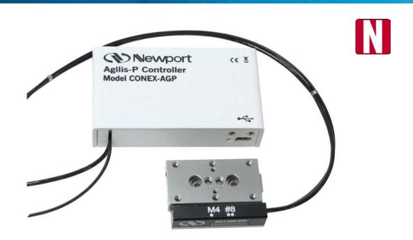
The CONEX-AG-LS25-27P is a piezo motor linear stage integrated with a closed-loop piezo motor controller/driver. For out-of-the box control, the CONEX-AGP controller is preconfigured and delivered with an Agilis AG-LS25-27P linear stage with a built-in direct read linear encoder.
