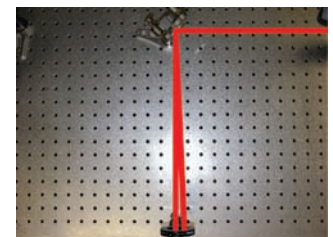
Figure 4.2 The iris should then be moved away from the 2nd routing mirror
