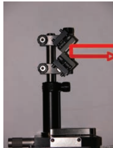
Figure 4.4 The beam exiting the delay line should travel parallel to the incoming beam
