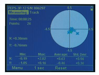
When connected to 1919-R power meter, the detectors also provide the beam tracking information such as the min and max Y/Y positions, average position, and standard deviation.
