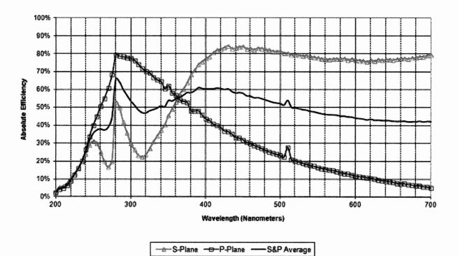
Note: The efficiency curve above is absolute and was measured in an in-plane near Littrow configuration (unless otherwise indicated). Efficiency curves are only representative: actual efficiency may vary significantly depending on use geometry and measurement technique. This efficiency curve is for master 6001; two masters with the same catalog number may have different efficiency curves. The uncertainty band on the data in the above efficiency curve(s) is +/- three percentage points.
