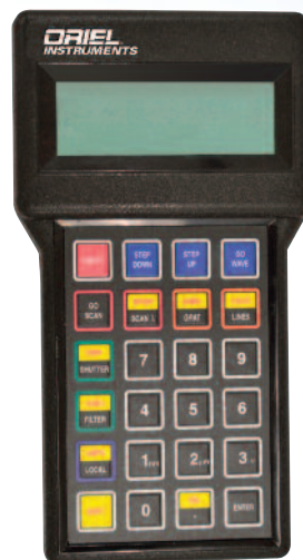
The Model 74009 optional hand controller is compatible with all Cornerstone 260 monochromators.
