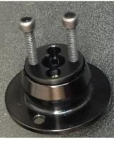
3. Insert the fiber adapter to 818-FA adapter holder. To achieve the most repeatable measurements, use the included screws to fasten the FP4-COL-1550, fiber adapter, and 818-FA.
