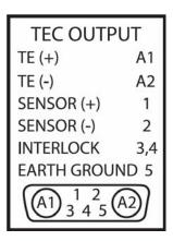
Figure 15 Pinout of cable for models 3150 and 3700
