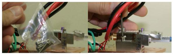
Figure 11 Mounting screws for BWA series LD
