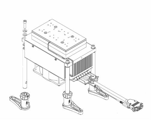
Figure 6 Model 764H-110 mounting hardware and electrical connections
