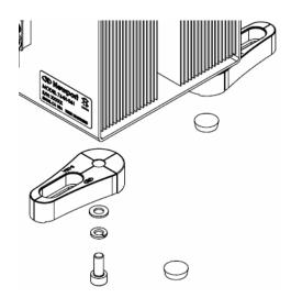
Figure 3 Model 764H-061 base mounting options. One can use either mount a B-05A slotted base for mounting on an optical table, or simply put a sticky rubber foot at each corner.
