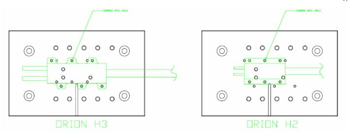
Figure 9 Hole patterns on 764H-061 top plate for Oclaro's Orion H2 and H3 package styles
