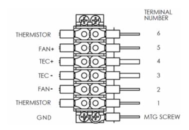
Figure 14 Terminal block connections
