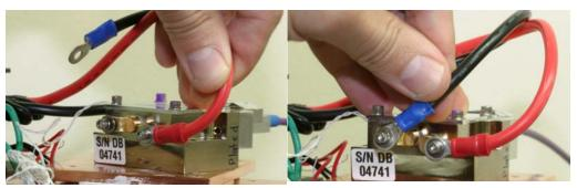
Figure 13 LD wire connections
