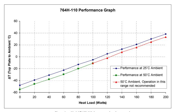
Figure 4 Model 764H-110 heat removal performance chart
