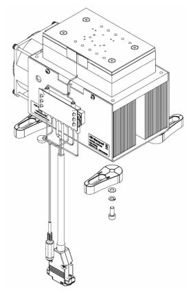
Figure 5 Model 764H-061 mounting hardware and electrical connections
