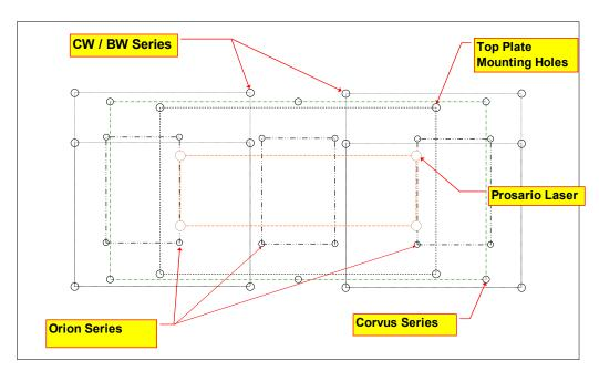
Figure 10 Hole patterns on 764H-110 top plate
