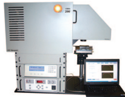
The Oriel IQE-AC family of automated solutions for measuring PV spectral response
