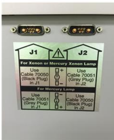
Figure 11 The label directing which electrical connector to use for each lamp housing interconnection cable on a 450-1000 W Research Lamp Housing.
