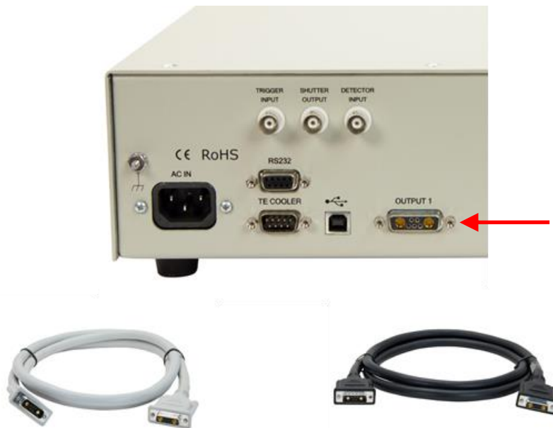
Figure 7 The output connector on the rear panel of the OPS-A150/OPS-A500 Power Supply for interface with Oriel Lamp Housing. The 70050 (Black) and 70051 (Grey) Lamp Housing Interconnection Cables are also shown.
