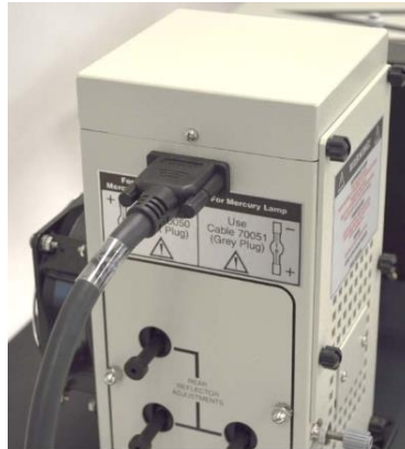
Figure 10 The electrical connector for interface with OPS-A Model Power Supply on an Oriel Research Lamp Housing.
