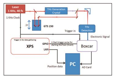
Fig. 2: Schematic of a THz scanning system (Courtesy of Fritz Haber Institute, Berlin, Germany)
