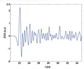
Fig. 4: THz signal versus time delay measurement (Courtesy of Fritz Haber Institute, Berlin, Germany)
