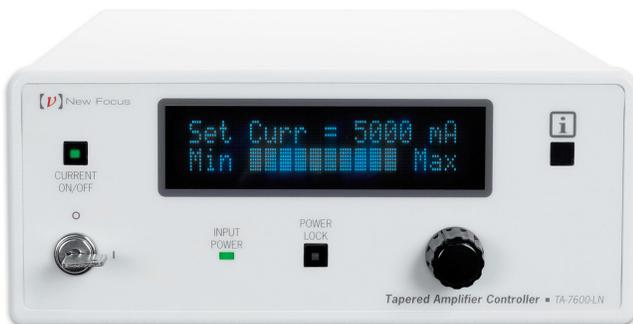
The VAMP TA is controlled using the TA-7600-LN Controller. Full control is made possible through the easy-to-use front panel interface. In addition, full control is also available using the USB or RS232 communication ports on the rear panel. Through the controller you can monitor the tapered diode temperature by way of a temperature sensor mounted on the diode block. Thermoelectric coolers are used to control the temperature of the diode.
