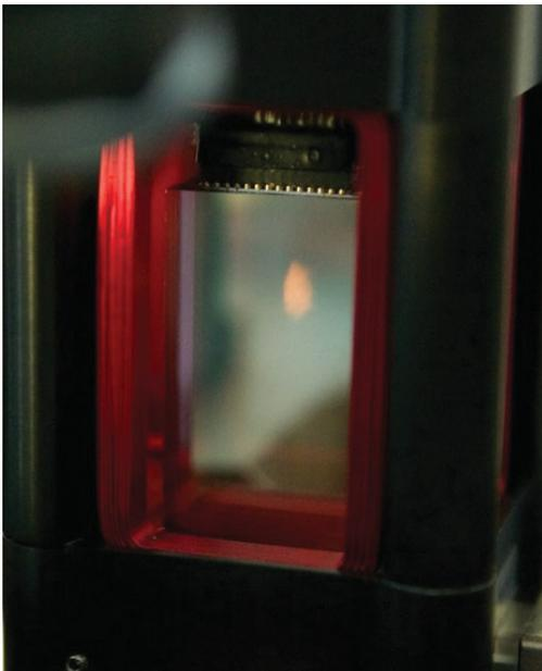
ColdQuanta's innovative BEC system is designed to streamline and simplify the production of ultracold atoms and BECs. At the heart of the system is the RuBECi® where rubidium atoms are cooled to temperatures of below 1  $\mu$ K, trapped, and manipulated inside the vacuum cell. A New Focus Tapered Amplifier is used to provide ample power for laser cooling and manipulation of the atoms.
