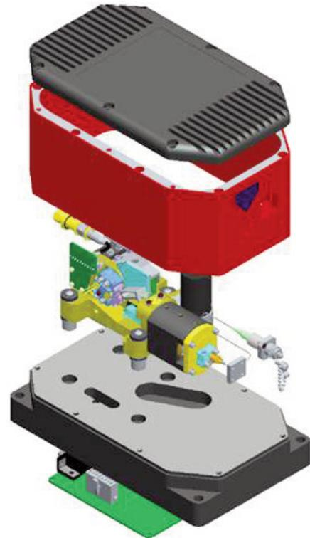
*Mechanical schematic of the TLB-6700 laser platform*
