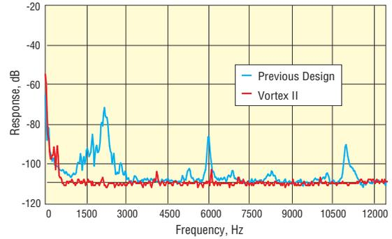
Frequency response of Vortex II in comparison with original Vortex (100 dB white noise test). The Vortex II has improved stability due to the Star-Flex design and magnetic damping.
