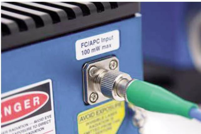
FC/APC input connector on the VAMP TA makes alignment a snap.
