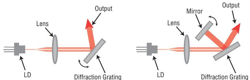
Figure 2: Tunable external-cavity diode lasers in Littrow and Littman-Metcalf configuration
