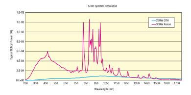
Photodetectors with NIST traceable calibration are used to measure the output power from 300-1650 nm from each unit manufactured. The results are part of the characterization report packaged with each system.
