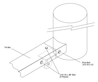
Figure 2.3 Assembling Tie-Bar to the Isolator
