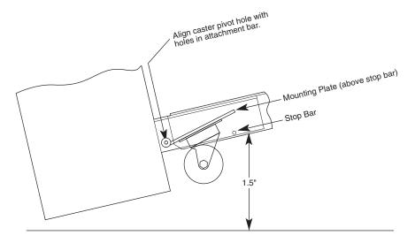
Figure 2.2 Installing Caster
