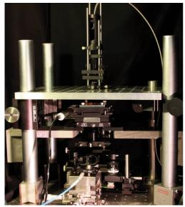
Figure 3: The experimental setup of Photonic Crystal Resonator Tester at Stanford, featuring stacked aperture stages with integrated actuators controlled by NSTRUCT (courtesy of Meredith M. Lee, PhD candidate)
