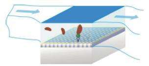
Figure 1: Sensing with a resonant photonic crystal slab
