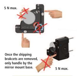
Do not apply excessive force on the mobile part of the mirror mount. The sensor is fragile and will be destroyed by such an action.
